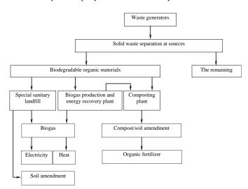
Fig. 4 A proposed solution for reuse and recycling of biodegradable organic domestic solid waste in HCMC.
